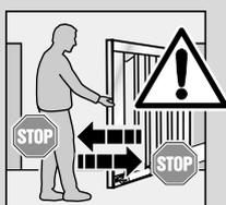
All persons using the gate system must be shown how to operate it properly and safely. Demonstrate and test the mechanical release as well as the safety return. To do this, halt the closing gate by grasping it with both hands. The gate system must initiate the safety return.
